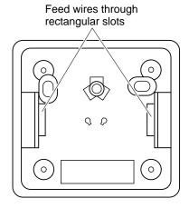
Figure 45 - Back View of Thermostat Base
